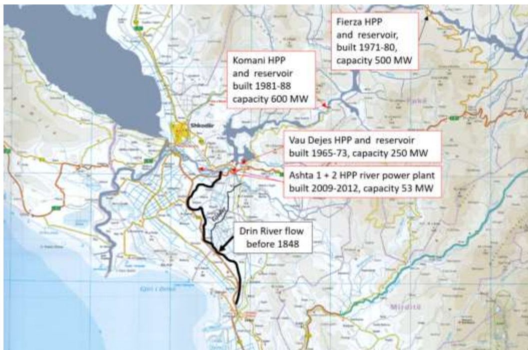
Figure 13: Flow of Drin and Gjadër River before diversion in 1848 and the Drin hydropower cascade including the river power plant Ashta (INFRASTRUKTUR & UMWELT, 2013)
